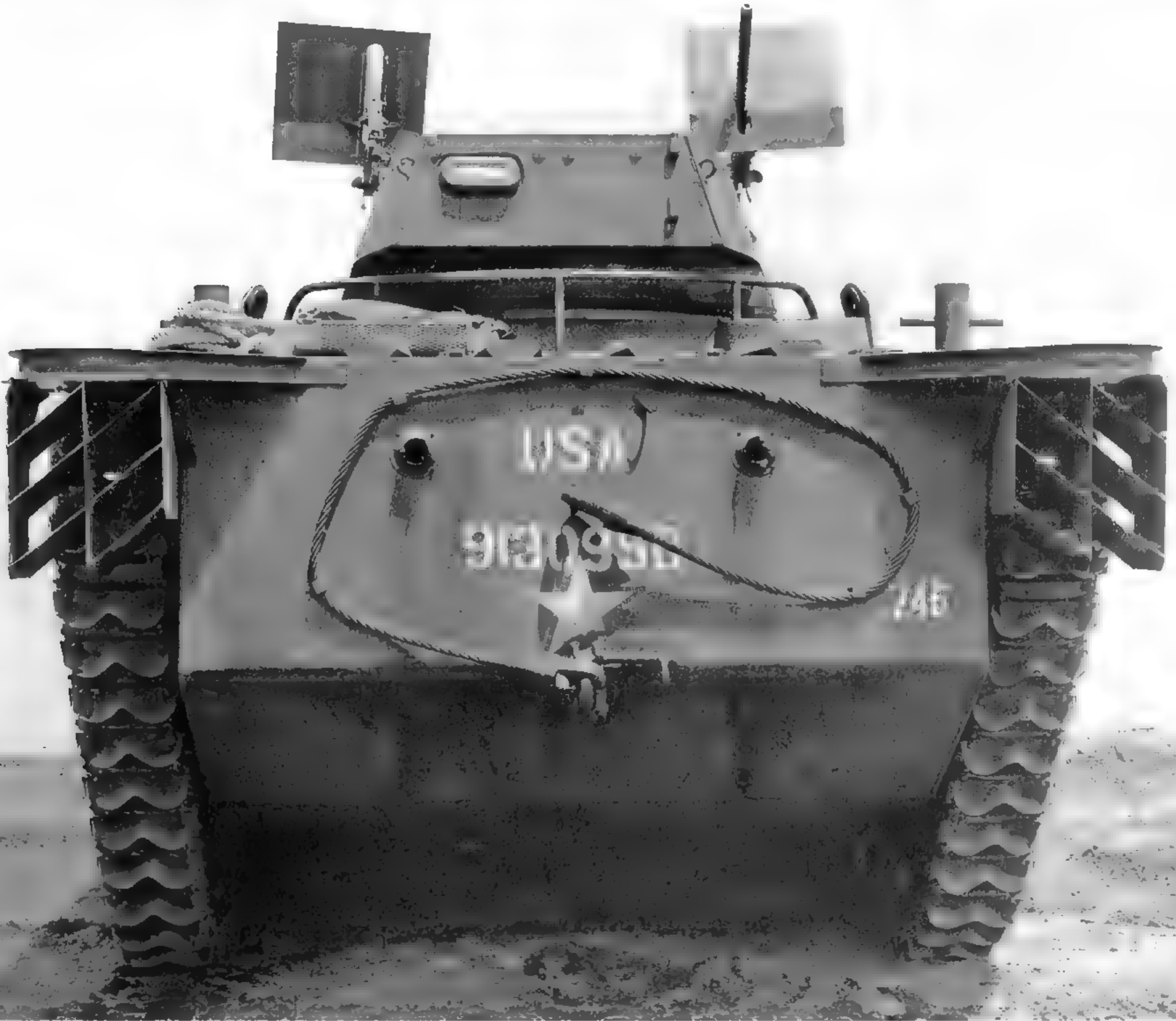
In addition to a turret basket to support the turret crew, another improvement in the LVT(A)5 was a vision block on the turret rear. (U.S. Army photo)
